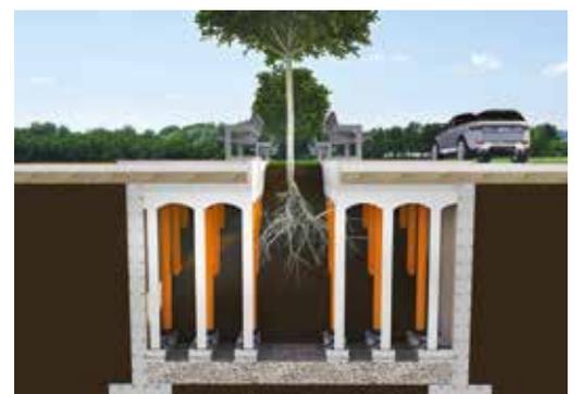
Section of New Elevator Root system
