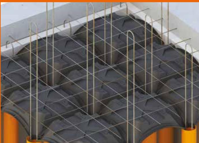
Place the wire mesh and the steel reinforcement in the pillars.
