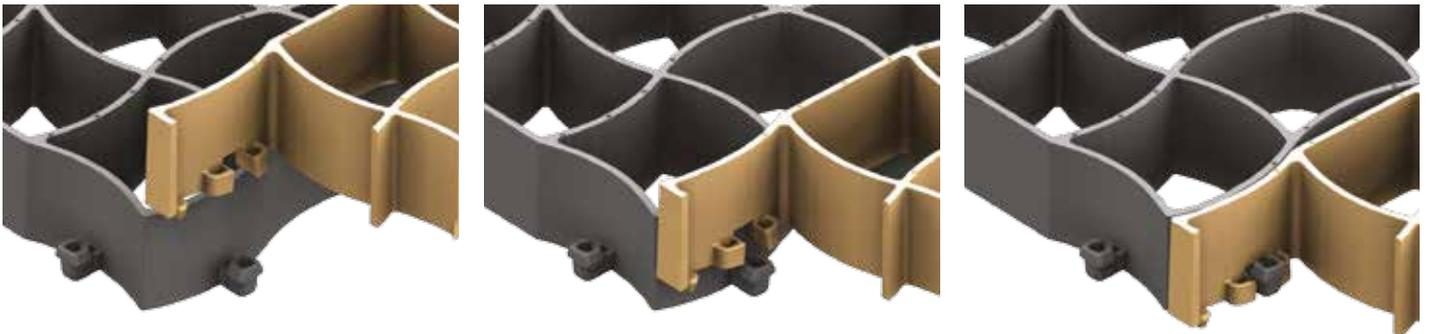
The innovative bayonet twist lock (male-female) simplifies installation and guarantees a perfect fixing of the grids. The characteristic *"Click"* indicates that the connection has been successful. It is possible and recommended to pre-assemble the elements of the grid before positioning it, in order to speed up the installation.
